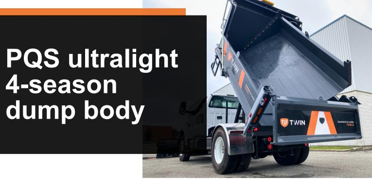
The new PQS ultralight 4-season dump body combines all the functionality of our popular 4-season but with the new Hardox 500 Tuff, which allows us to reduce the weight of the body by 600 lb while increasing its capacity by ½ cubic yard.
